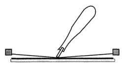
Off contact is particularly important when printing nylon that is lined with either quilt or fleece. Jackets that are lined with these fabrics should have approximately 1/16" off contact. Excessive off contact requires extra squeegee pressure causing the same slurring or double imaging. The thickness of these linings will cause the garment to retain heat longer than thinner lined or unlined garments.
